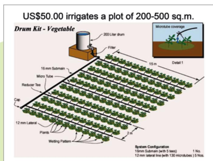
A typical 200-litre mini-tank (drum) LHLCD irrigation system.
